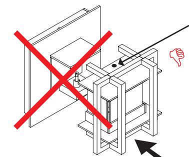
The screw hole at the bottom side.
